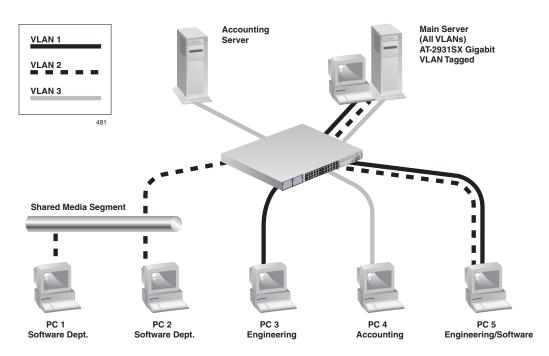
Figure 34. Example of Servers Supporting Multiple VLANs with Tagging
